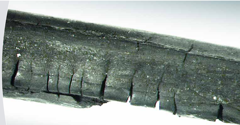
Extreme thermal stress on an O-ring
