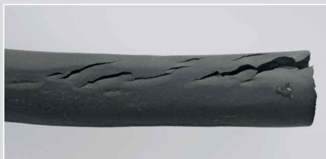
Enlarged view of a conventional sealing ring, which exhibits clear signs of damage as a result of explosive decompression.
